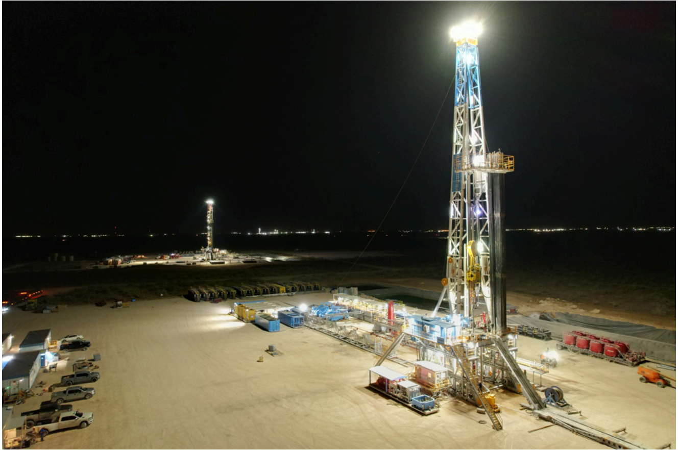
Fig. 1. In this image taken with a drone on the night of Aug. 21, 2024, Latshaw Drilling Rig 19 works for Double Eagle Energy Holdings IV, LLC, in the Permian basin. The 1,500-hp rig was working on its first pad for that operator and had walked 120 ft out from its original well. Image: Latshaw Drilling.
