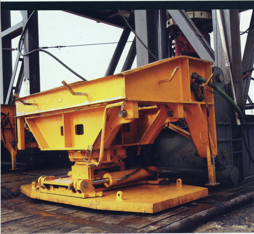
Above, a close-up view of the NOV Steeltoe hydraulic jack walking system on Latshaw Rig 42, also pictured at right. The walking system allows the rig to move in any direction on a multiwell pad.
